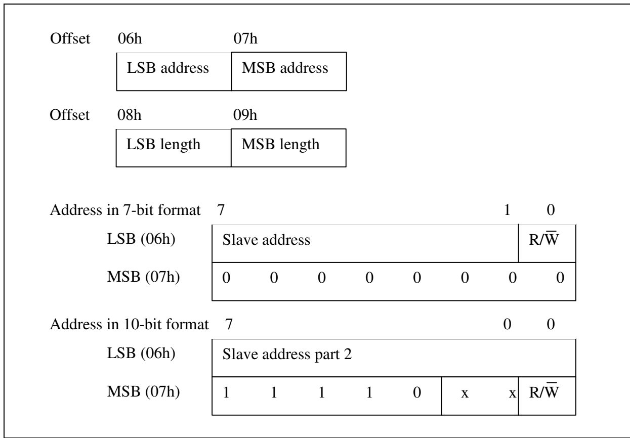
Chart 3-13: Telegram data for OP_ANAGATE_I2C_READ_REQ
